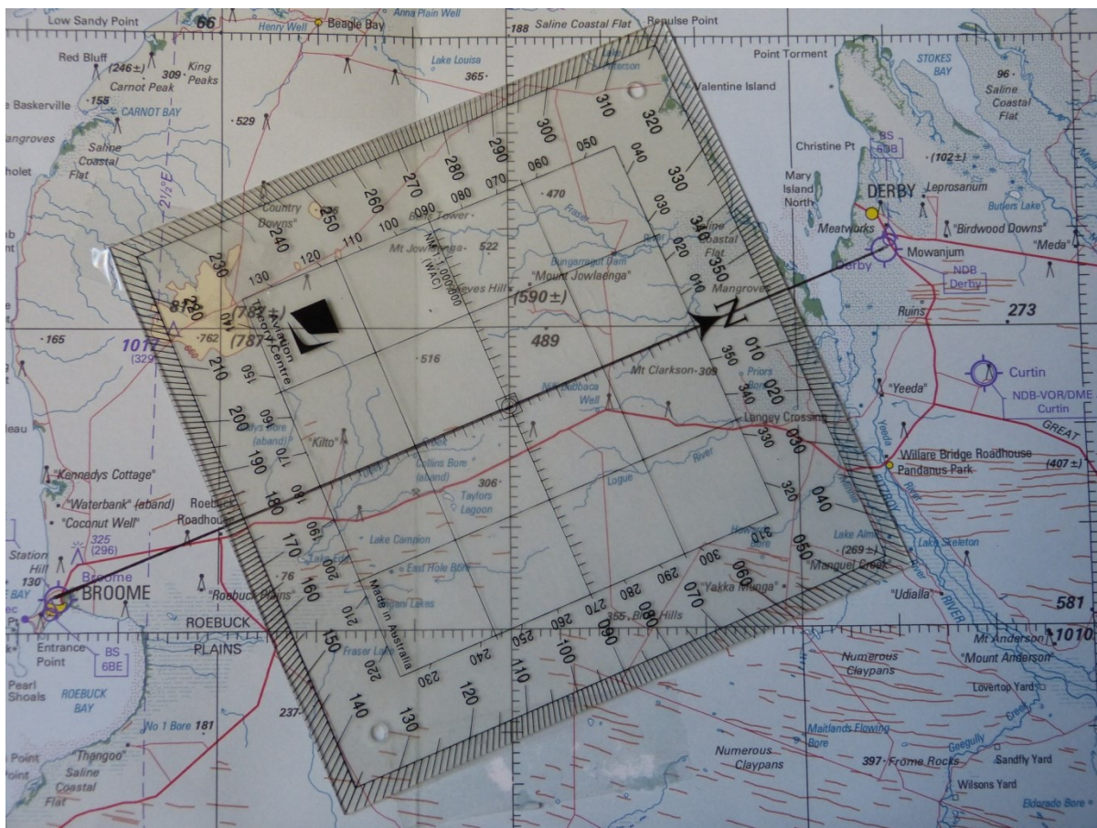
Fig. 11 An alternative way of measuring a track angle
