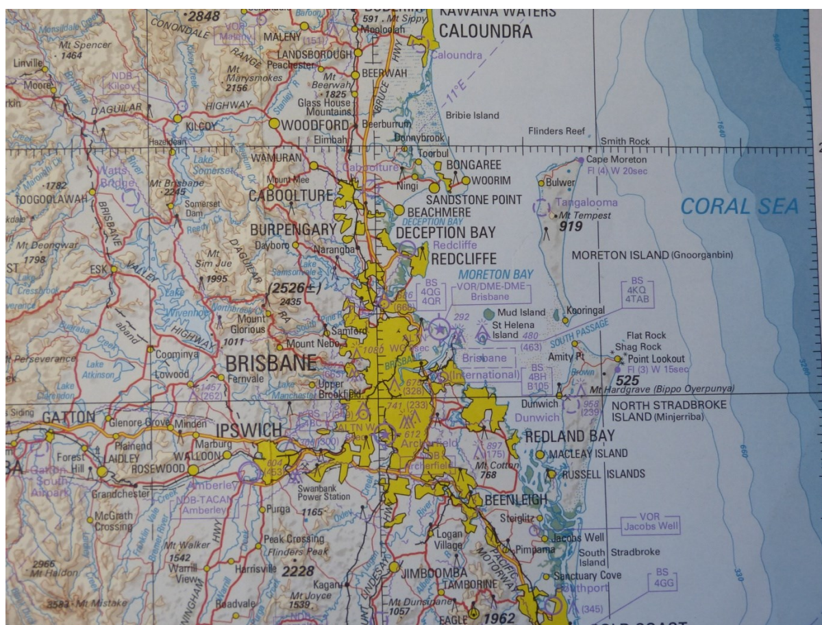
Fig. 9 Information for visual navigation as it appears on a World Aeronautical Chart
