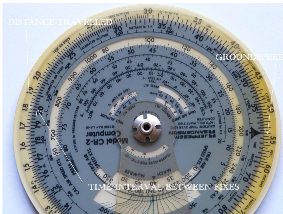
Fig. 34 Using the slide rule to calculate ground speeds
